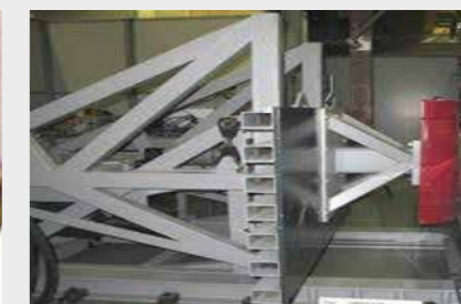
Intrusion test 200kN
